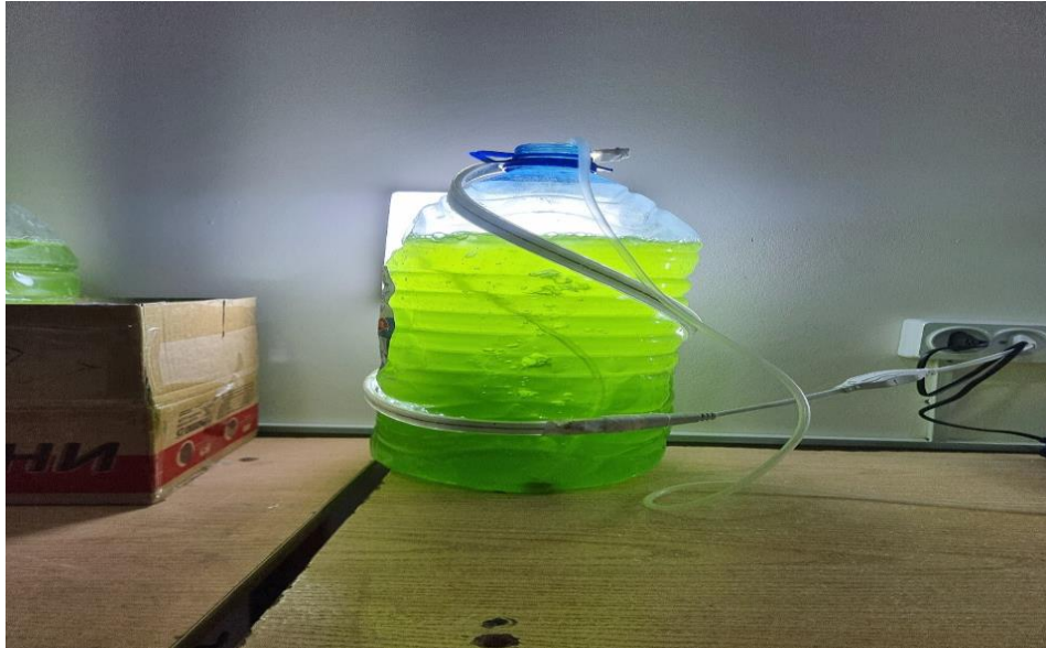
Figure 1. Laboratory-scale cultivation system used for producing Chlorella vulgaris liquid culture applied in the mushroom cultivation experiment.
