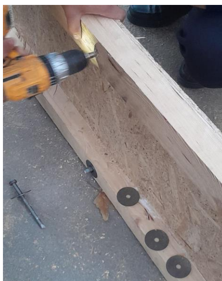
Figure 3. Use of bolted connections during the fabrication of the timber beam model
