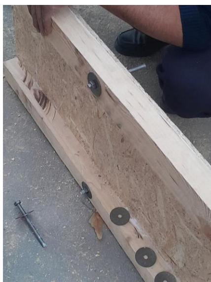
Figure 3. Use of bolted connections during the fabrication of the timber beam model
