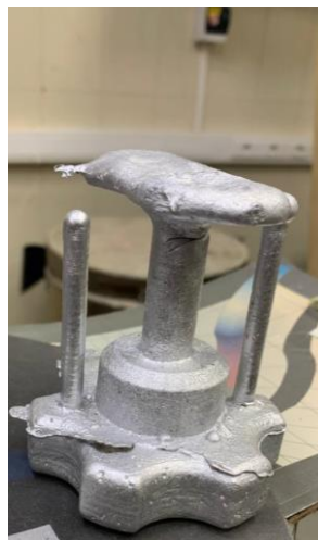
Figure 2. Final aluminum casting with gating system and feeder. (Insert photo of the finished casting after mold removal.)
