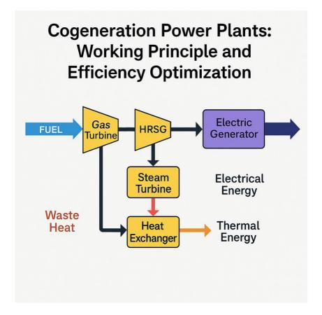
This study aims to examine the core working principle of cogeneration systems, their technical infrastructure, and efficiency characteristics. It also highlights real-world applications, compares them with conventional systems, and explores how cogeneration contributes to broader energy and environmental policy goals. Ultimately, this paper underscores the relevance of cogeneration in building a resilient and low-carbon future energy landscape.
