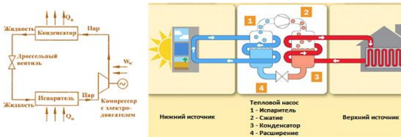
Figure 1. Structure and Operating Principle of a Heat Pump
