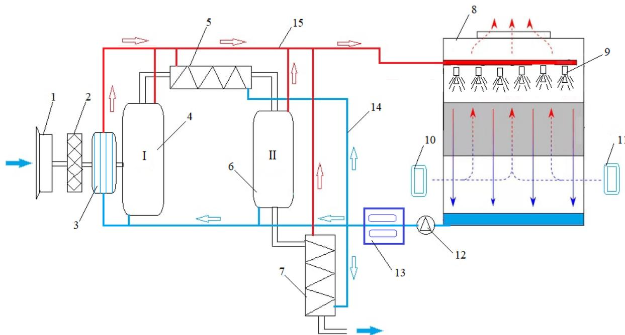
**Fig.7. Schematic diagram of the open-circuit cooling system of a two-stage reciprocating compressor after modernization.**
