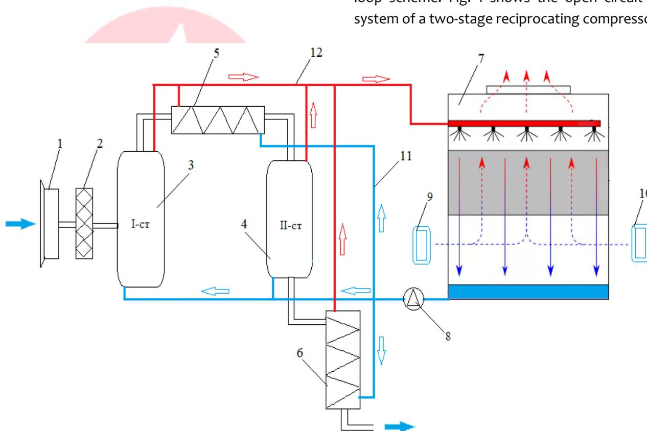
Fig.1. Schematic diagram of the open-circuit cooling system of a two-stage reciprocating compressor.
