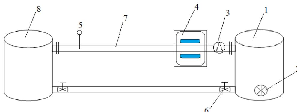
Fig. 4. Schematic view of the experimental setup when testing the device for electromagnetic water treatment.
