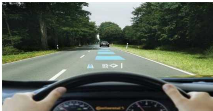
Fig. 9. Head -up display (HUD)
