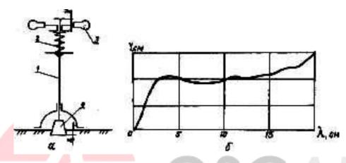
the form of a diagram (Fig. 1-a). The ordinate Y of the diagram indicates the amount of compression of the spring, and the abscissa (indicates the depth of penetration of the triple into the soil. If the compression caliber of the spring is Kn (n/cm), the resistance of the soil to the penetration of the triple is calculated as R q KnY.
