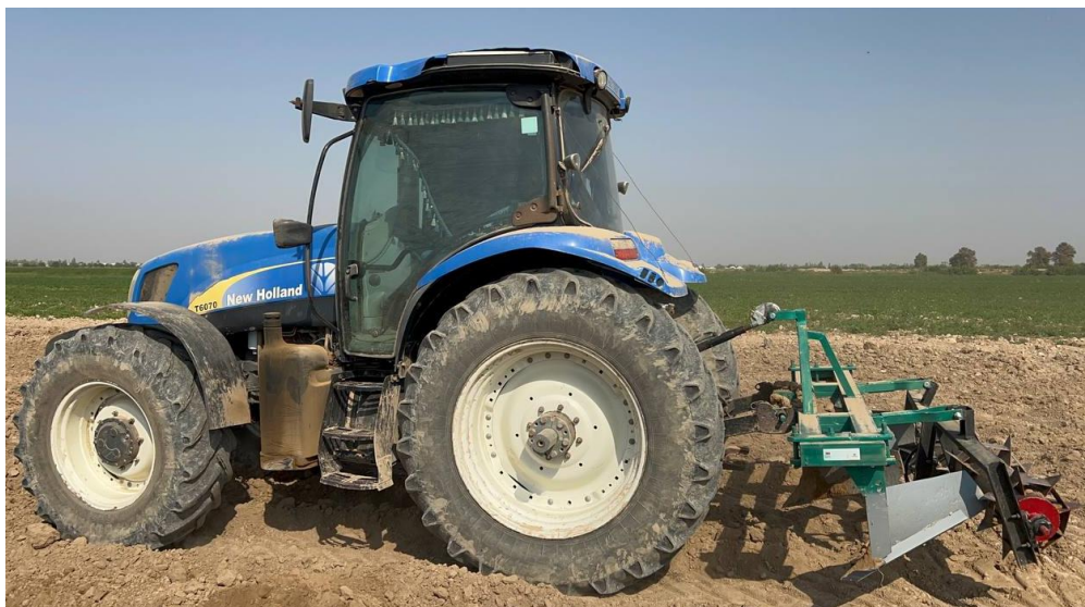
Figure 1. Side view of the ridge-forming machine equipped with a crumpling roller
